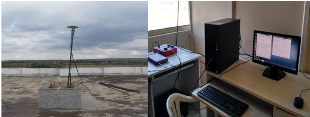
Figure 1. Septentrio PolaRxs-Pro GNSS receiver and antenna setup at GCET, Hyderabad
